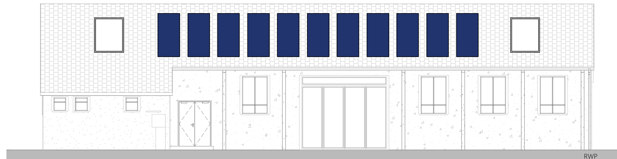
Proposed North-West Facing Elevation Scale 1 : 100
